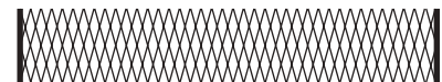
Common Flexible Hose is Weak and Loosely Knit and can't be used in High Pressure
